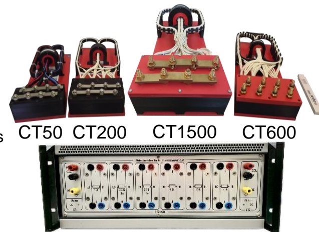
Figure 2: The accomplished wideband current-to-voltage transformer set for currents up to 2 kA. The symmetrical current transformers (above) and the front panel of the associated precise measuring resistor box (below)
