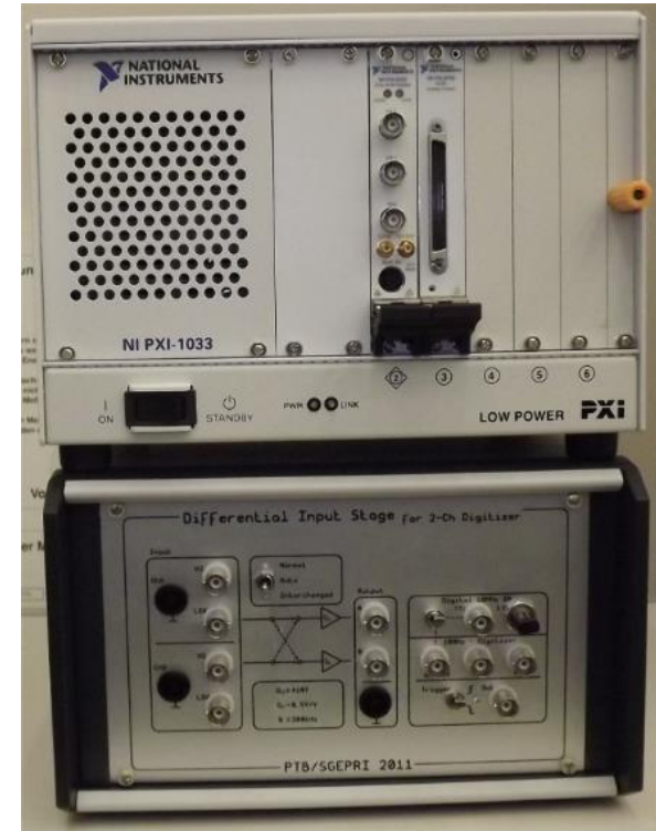
Figure 3: Photo of the 2-channel precision ratio measuring system ( VRS)
