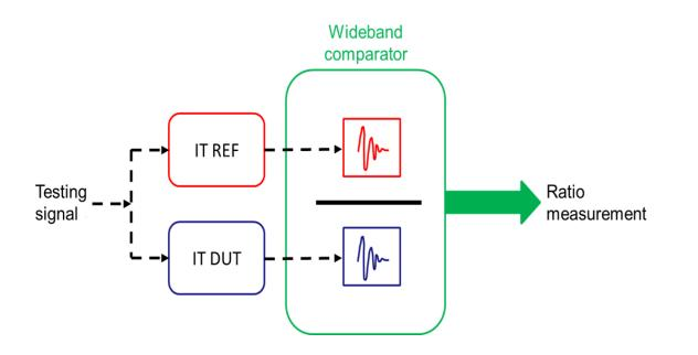
used to compare the outputs of ITs
